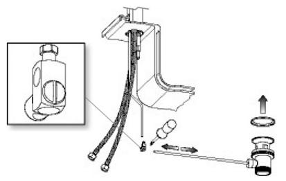
9. Connect the hot and cold feed pipes to the supply pipes using the appropriate sized compression fittings (not supplied)
